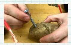
Connect the two potatoes together with the wire going from the penny to the screw.
